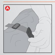
Release safety straps, and unroll cover over pickup bed. Open tailgate.
