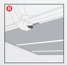
Roll up cover. **Do Not** disengage loop and hook fasteners prior to rolling up cover.
