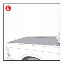
Pull cover tight across width of pickup bed. Secure loop and hook fasteners on opposite side rail.
