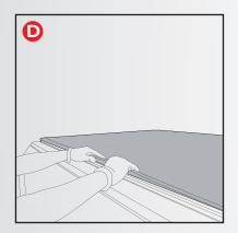
Secure loop to hook fasteners on one side rail by pressing edge of cover along full length of rail.
