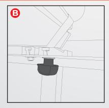
With tailgate open, hook tailgate header into header stops on both sides of vehicle.
