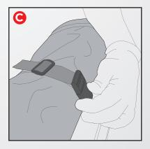
Always secure cover at front of pickup bed with both safety straps when cover is open.
