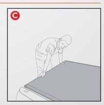
Rotate tailgate header down until both latches engage. Listen for double click
