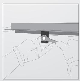
**2.** Set cover assembly on front bulkhead and insert the screws into the holes of the side rails like the picture.
