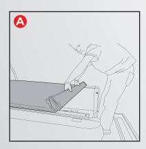
With tailgate open, press downward on cover and turn the knob underneath.
